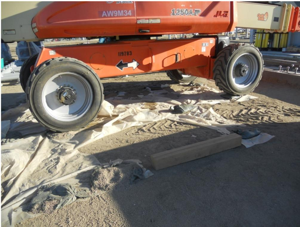
**Figure 3:** Improper secondary containment underneath equipment in Whirlwind Substation, Segment 9.
