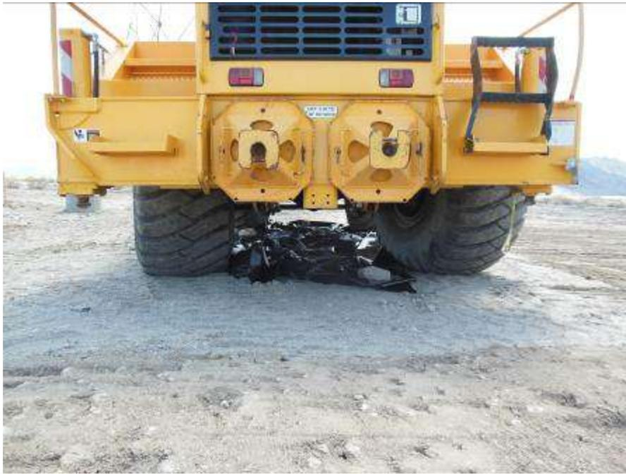
**Figure 7.** Plastic sheeting used for inadequate secondary containment at Tower RB2-3E.
