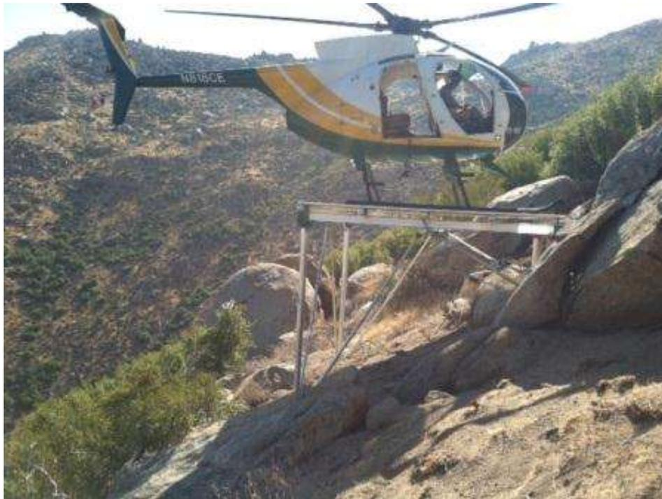
**Figure 6.** The new location of the temporary landing platform at Tower 1043. The location is just east of the permanent platform location and within the ROW boundaries.
