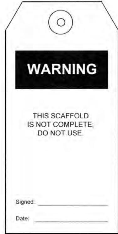
A rectangular scaffold tag with a circular hole at the top center. A black horizontal bar at the top contains the word "WARNING" in white. Below the bar, the text reads: "THIS SCAFFOLD IS NOT COMPLETE; DO NOT USE." At the bottom, there are two lines for "Signed:" and "Date:".
