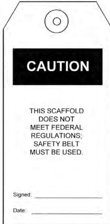
A rectangular scaffold tag with a circular hole at the top center. A black horizontal bar at the top contains the word "CAUTION" in white. Below the bar, the text reads: "THIS SCAFFOLD DOES NOT MEET FEDERAL REGULATIONS; SAFETY BELT MUST BE USED." At the bottom, there are two lines for "Signed:" and "Date:".
