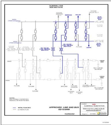
Figure 2.1.2-1. Schematic Single Line for Solution #1 Source: SCE
