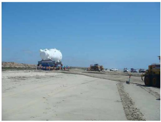
**Figure 3:** The RSG at a layover area above the mean high tide line along the beach route. The RSG was staged overnight in the layover areas and resumed transport during the next low tide. Ramps created for RSG access/egress were re-contoured after use.
