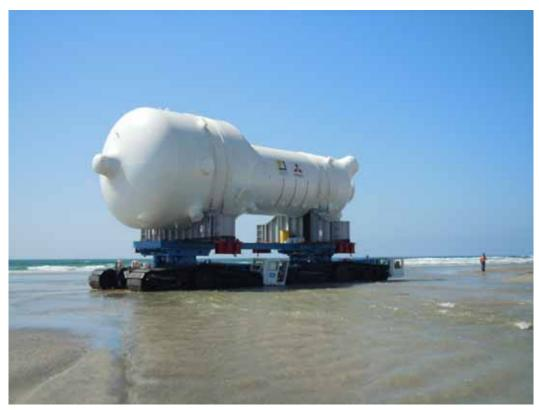
**Figure 1:** RSG on the crawler crossing the Santa Margarita River along the beach route on MCBCP.
