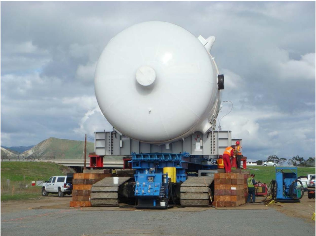
**Figure 7:** The crawler in position at Las Pulgas to offload the RSG and transfer onto the Goldhofer, which will be used to take the RSG to the SONGS facility.
