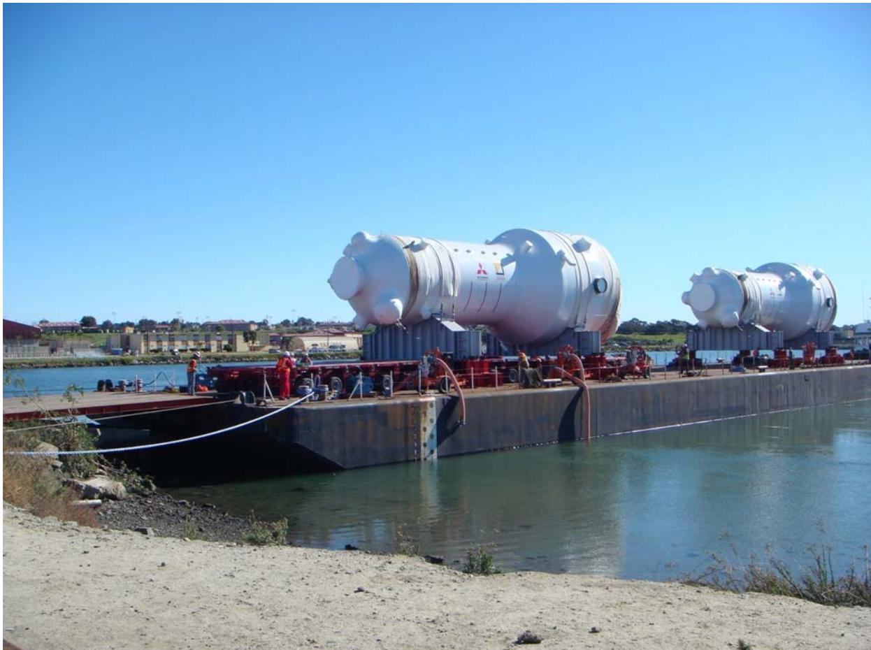
**Figure 1:** A series of heavy lift transport trailers called a Goldhofer (red multi axle trailer) was driven onto the transport barge to offload each of the RSGs upon arrival to the Del Mar Boat Basin January 10, 2009.
