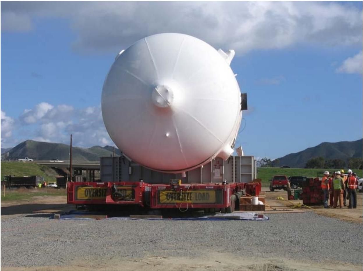
**Figure 8:** Transition to the Goldhofer at Las Pulgas staging area for transport along Interstate 5 and Old Highway 101 into the SONGS facility, scheduled to begin Wednesday night, January 28, 2009.
