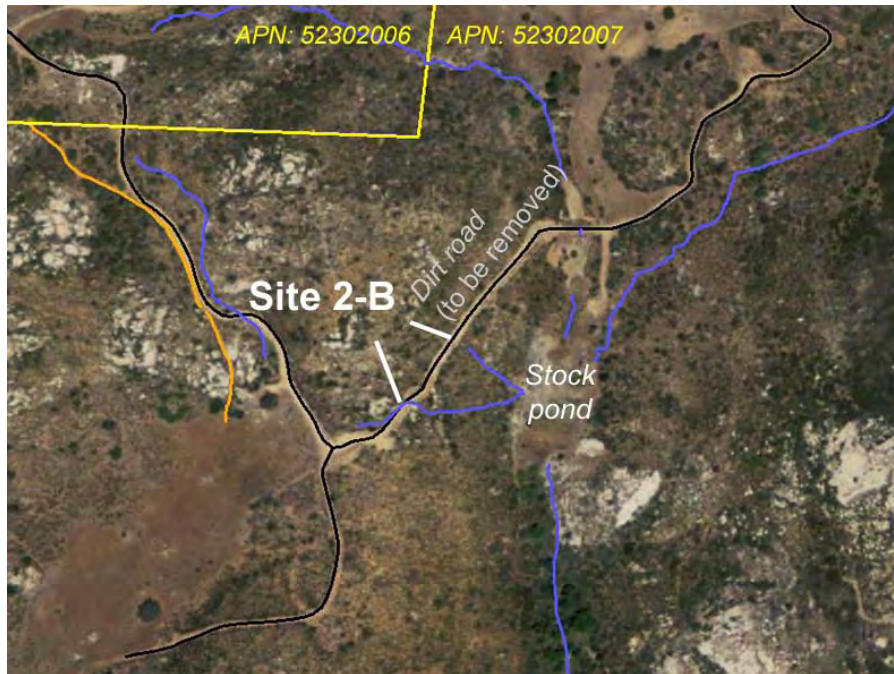
Figure 22. View of existing road crossings at Site 2-B along two ephemeral stream channels that drain eastward to the large stock pond (aerial photograph taken 25 May 2009, source: Google Earth, accessed 2010). Present day road alignment shown in black and streams shown in blue.
