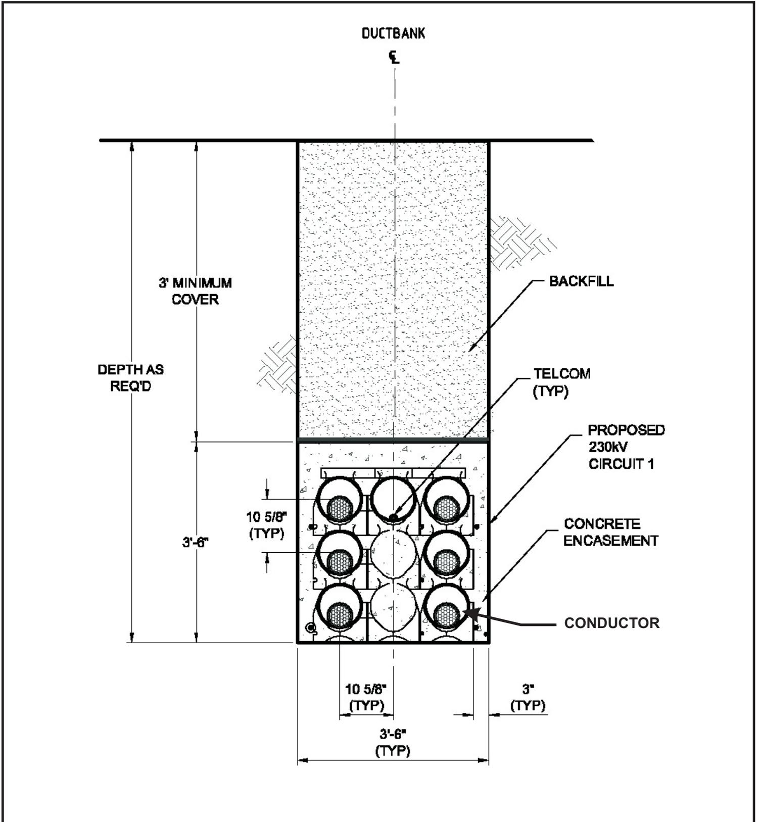
Note: There would be two adjacent trenches with duct banks for the DC 230 kV segment (Inland Valley) and one for the SC 230 kV segment (Coastal).
