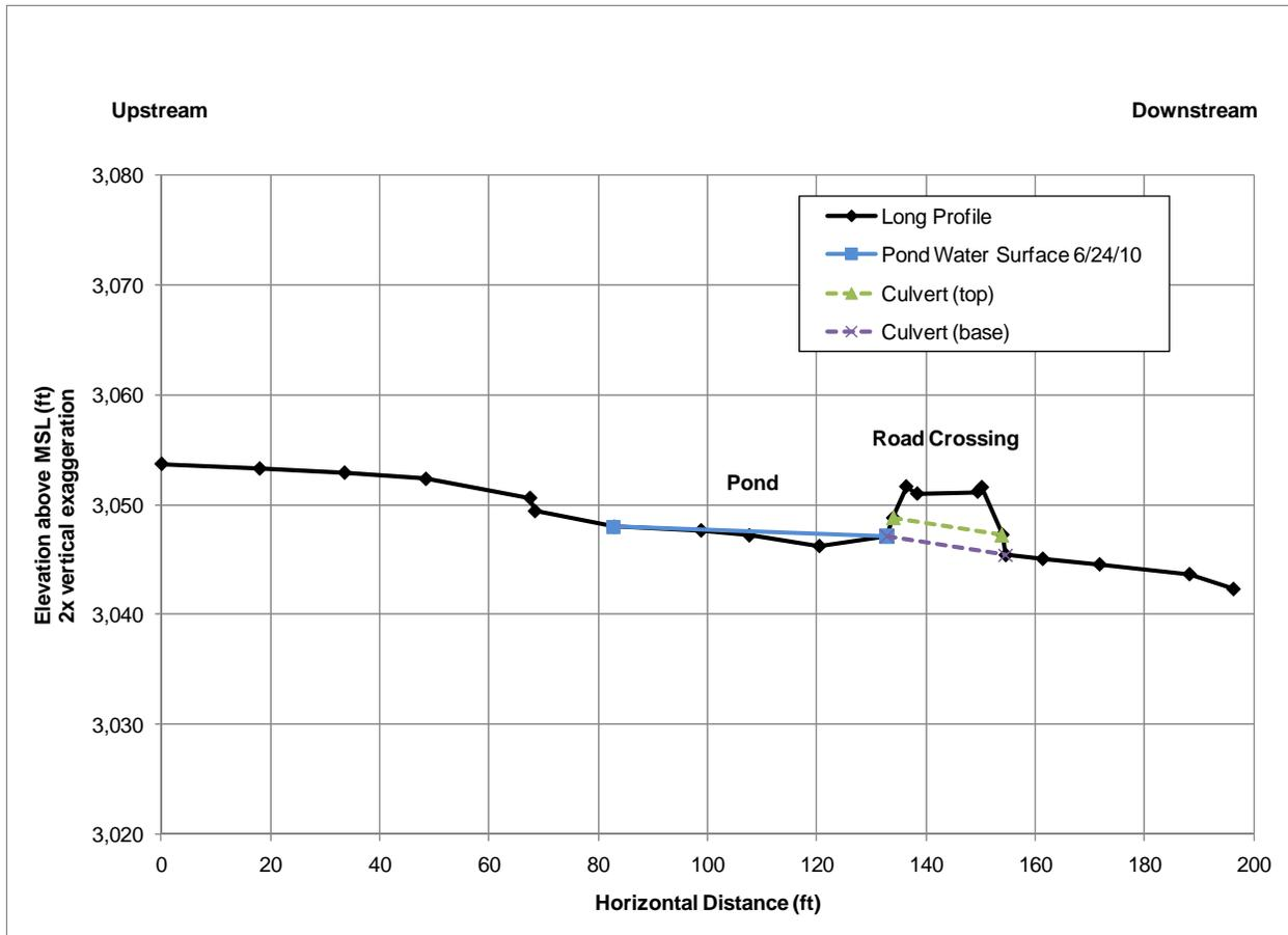
Figure C-6. Longitudinal profile along the intermittent stream channel at Site 1, with flow moving downstream from left to right. The road crossing presently impounds water on its upstream side forming a seasonal pond with wetland vegetation.
