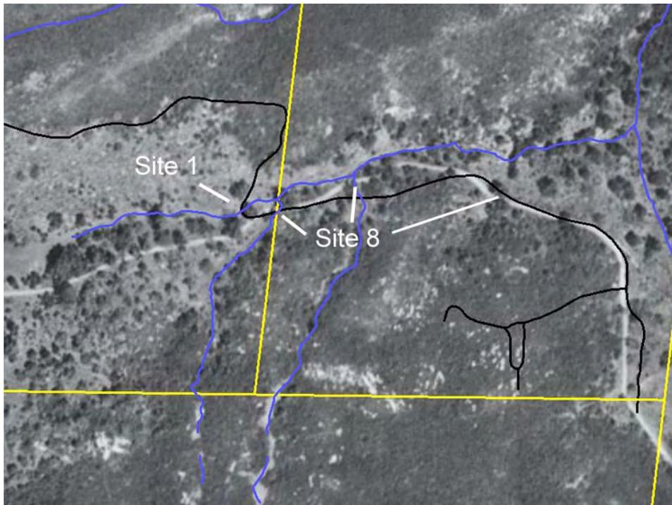
Figure C-2. View of historic road alignment at Sites 1 and 8 (aerial photograph taken 2 Apr 1953). Present day road alignment shown in black and streams shown in blue. Note that a road did not cross the stream at Site 1 (constructed 2002-2003) but did cross the three ephemeral tributary streams at Site 8.
