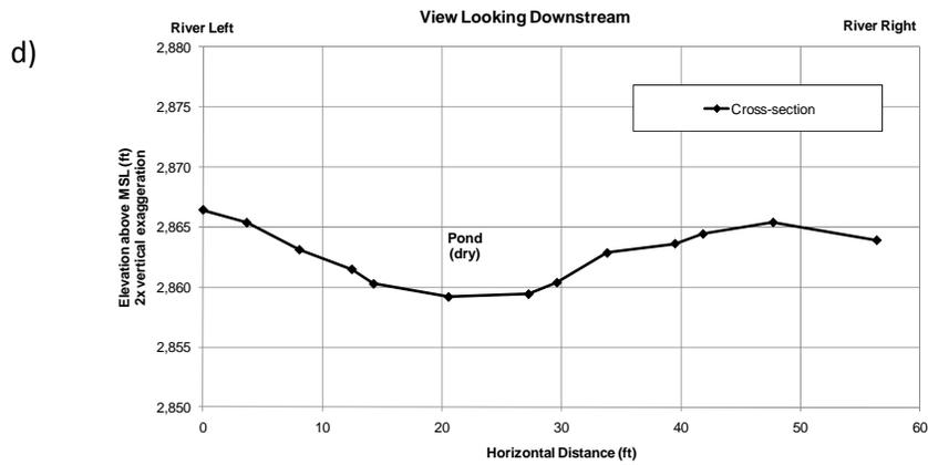
Figure C-29. Cross-sections along the northeastern stream channel above the large reservoir. The cross-sections span the natural stream channel above NE Pond A (a), the NE Pond A (b), the NE Pond B (c), and the NE Pond C above the large reservoir (d).
