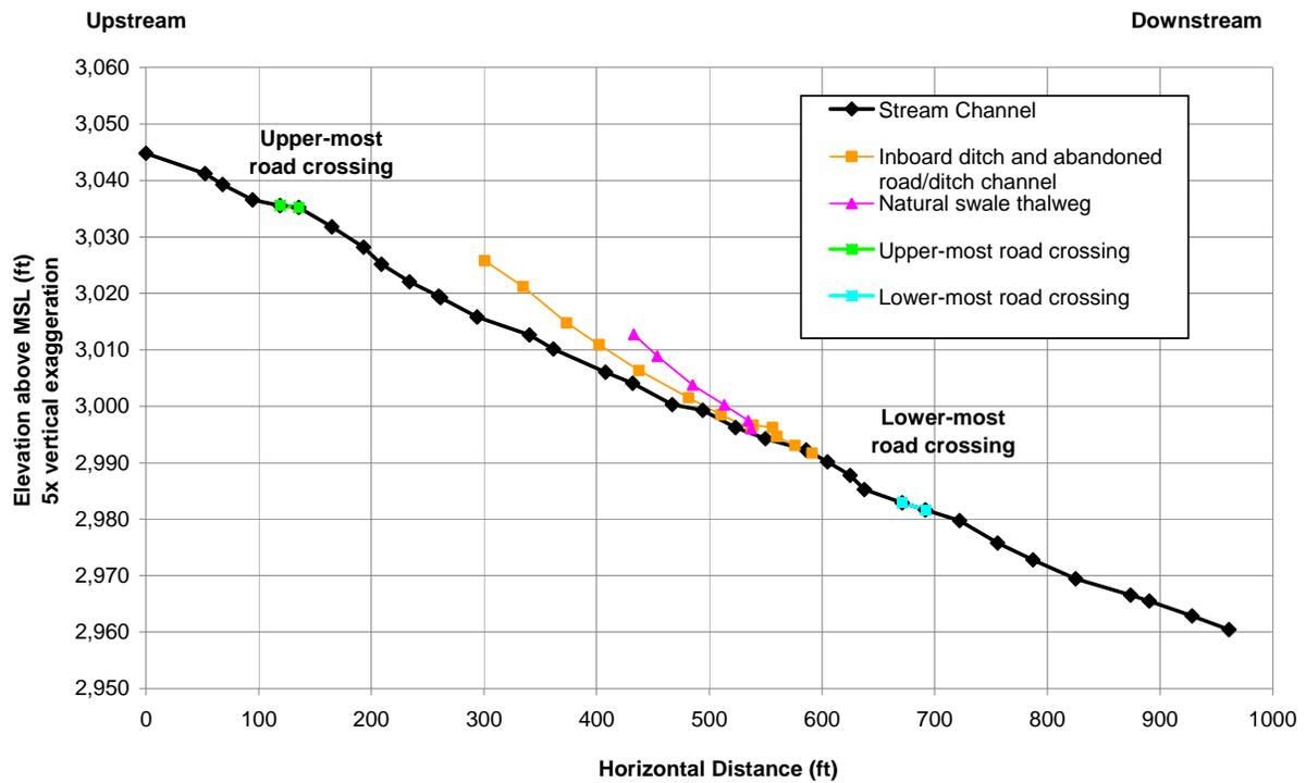
Figure C-15. Longitudinal profile along the intermittent stream channel at Site 1, with flow moving downstream from left to right. The road crossing presently impounds water on its upstream side forming a seasonal pond with wetland vegetation.
