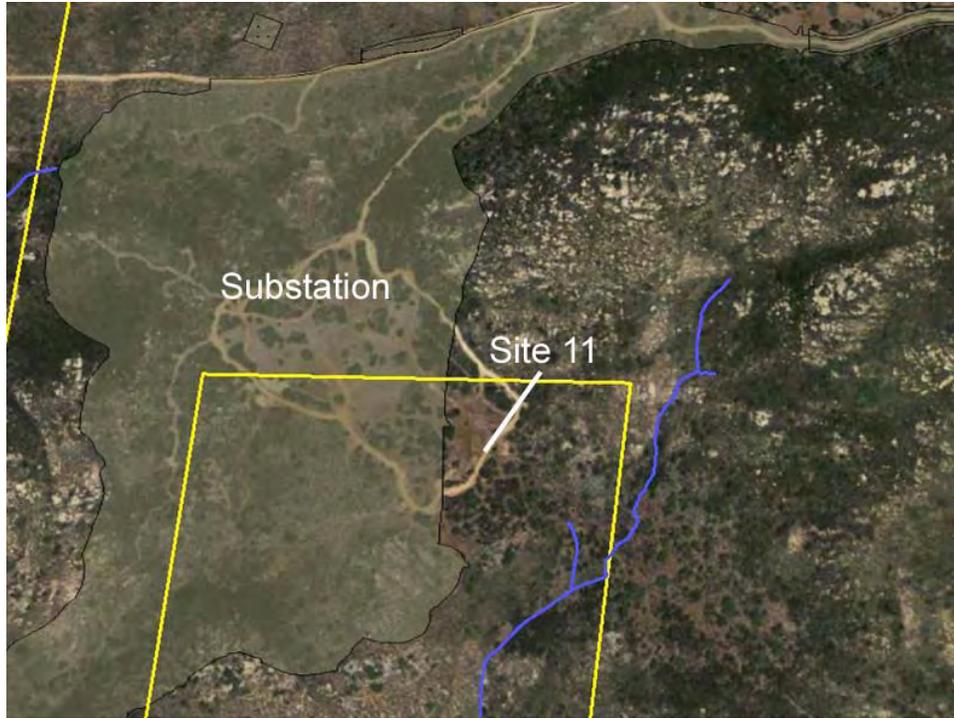
Figure C-20. View of existing road crossing at Site 11 above an ephemeral stream channel and situated on the east-side of the substation (aerial photograph taken 25 May 2009, source: Google Earth, accessed 2010). Present day road-loop alignment seen in the aerial photograph and streams shown in blue. Flow direction is to the southeast from the Site 11.
