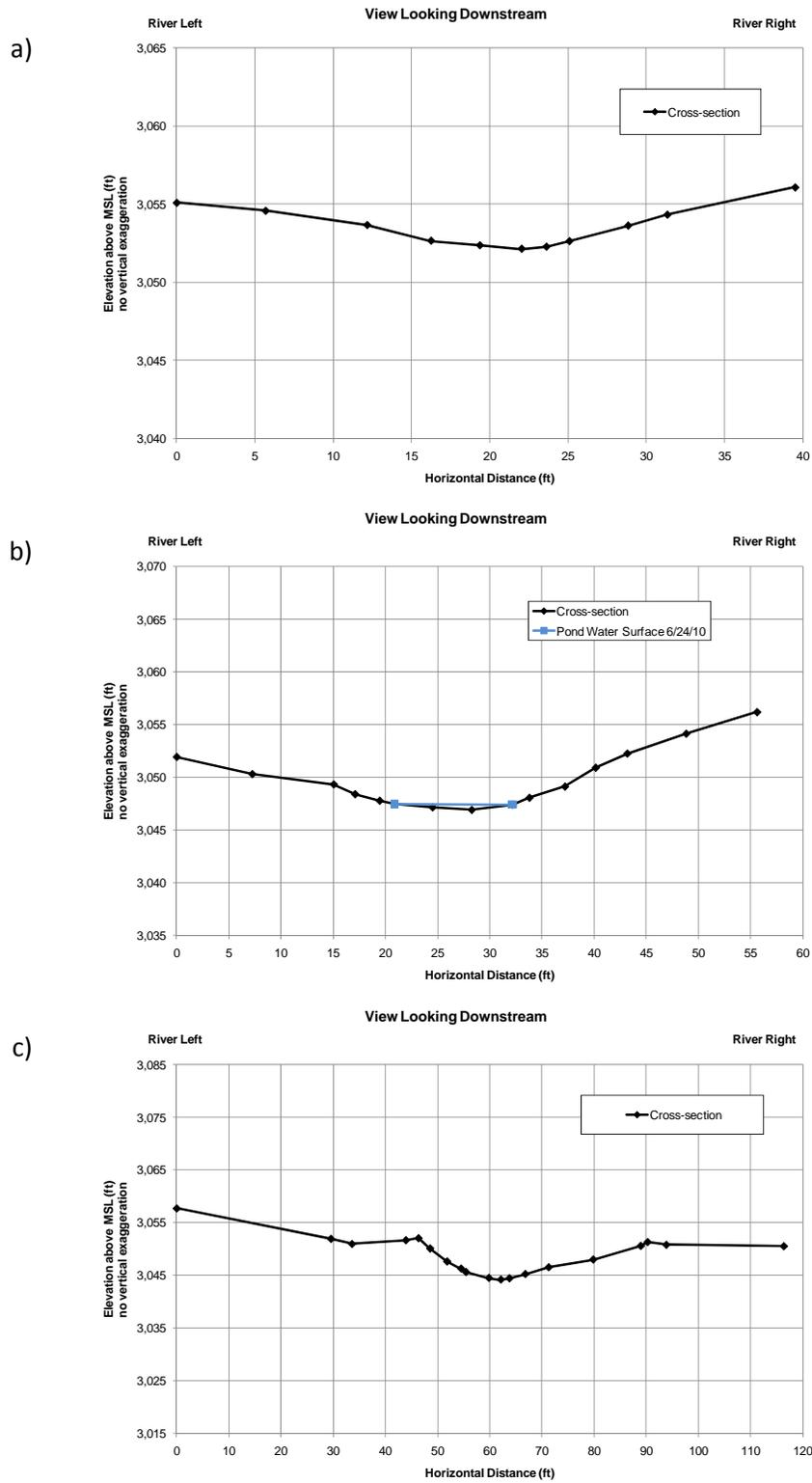
Figure C-5. Cross-sections upstream of the road crossing (a), across the pond upstream of the crossing (b), and downstream of the road crossing (c).
