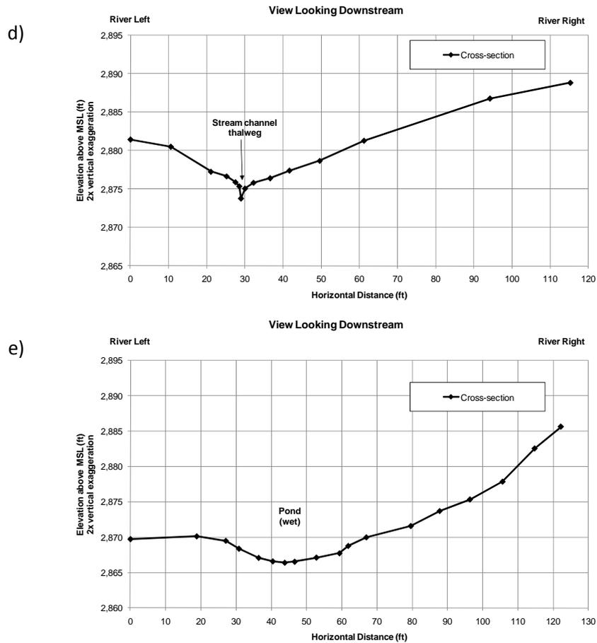
Figure C-28. Cross-sections along the northwestern stream channel above the large reservoir. The cross-sections span the natural stream channel above NW Pond A (a), the NW Pond A above the road crossing (b), the NW Pond B below the road crossing (c), the stream channel between NW Pond B and NW Pond C (d), and the NW Pond C above the large reservoir (e).
