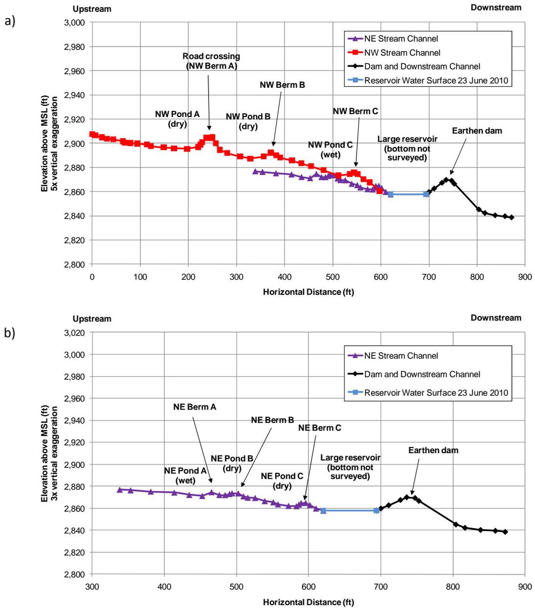
Figure C-27. Longitudinal profile along two intermittent stream channels that drain into the large reservoir at Site 3, with flow moving downstream from left to right (a). The longitudinal profile along the northeastern stream channel is shown as reference in (a) and alone in (b).
