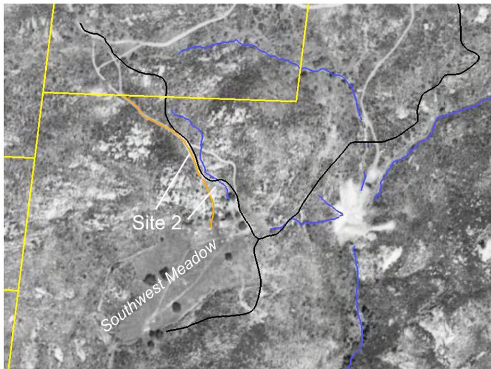
Figure C-10. View of historic road alignment at Site 2 (aerial photograph taken 2 Apr 1953). Present day road alignment shown in black, present day abandoned road and ditch shown in orange, and streams shown in blue. Note the abandoned road and ditch once served as the primary roadway.
