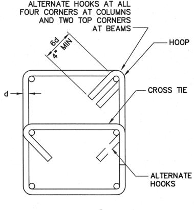
MAX SPACING = 12" AT SEISMIC TIES UNO COLUMN & BEAM TIE MAX SPACING = 12"
