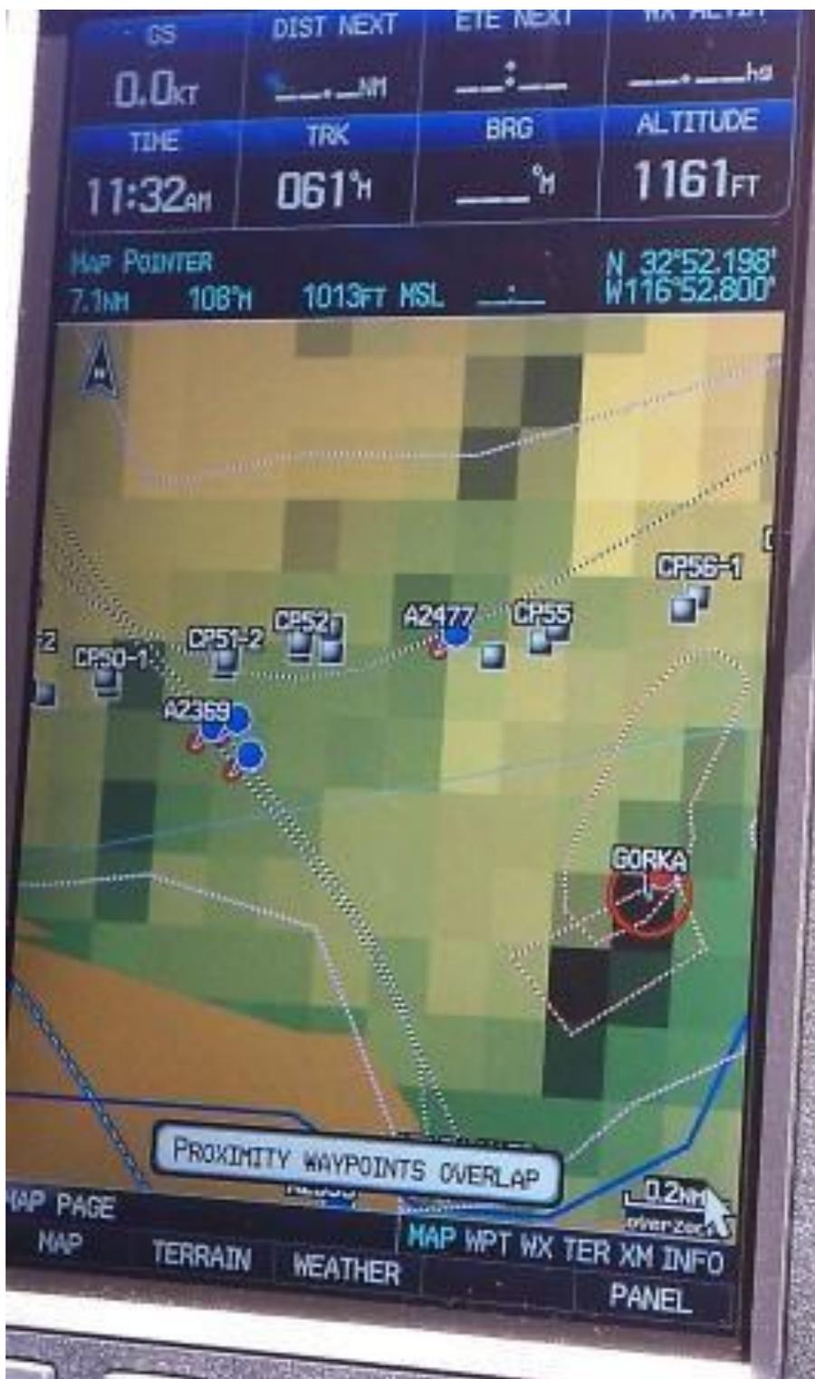
GPS unit display in helicopter showing tracks to Helix Yard and avoidance of sensitive areas.
