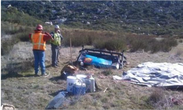
*Photo 39: Air compressor destroyed after falling from helicopter into a field.*
