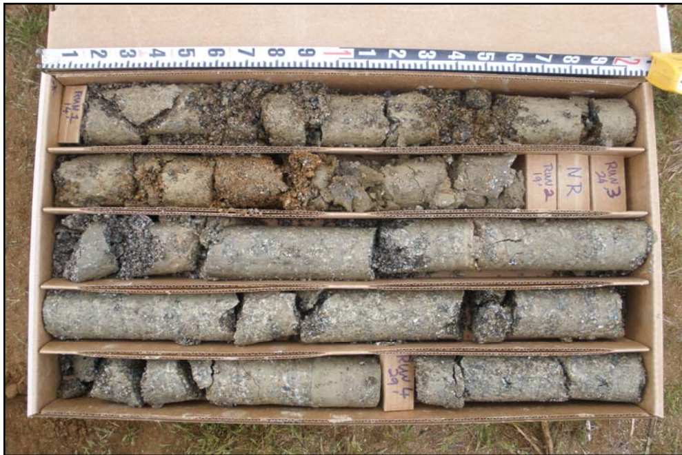
Boring CP-1, Depth Interval 14.75 to 30.0 ft bgs (Elevation 1116.75 to 1101 feet MSL)
