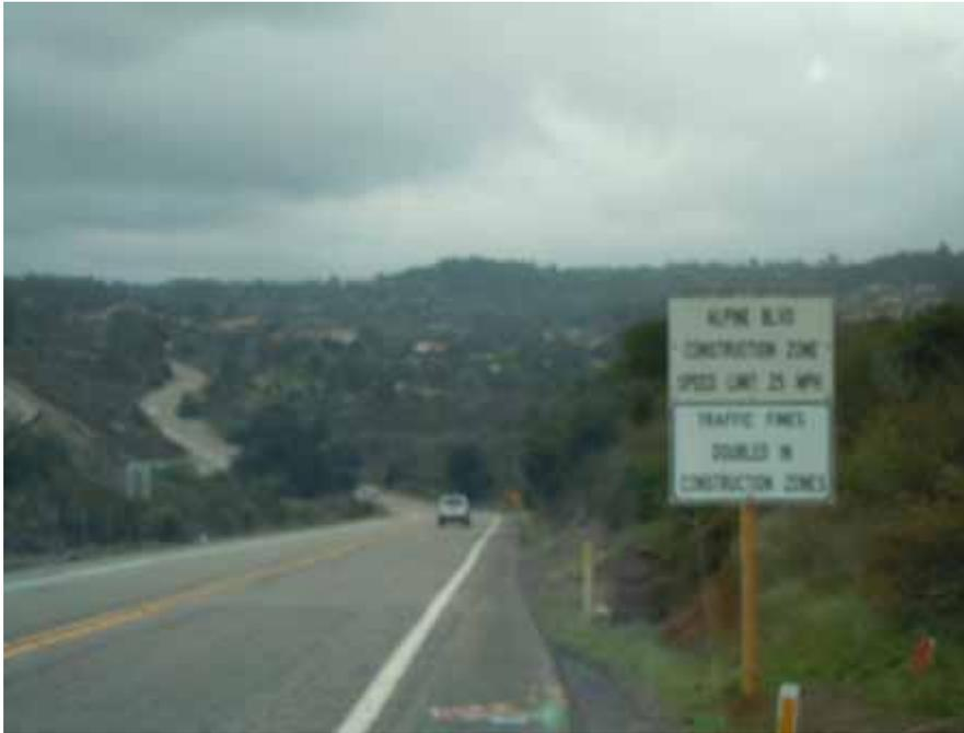
**Figure 1:** Posted signs along Alpine Boulevard per the San Diego County approved Traffic Control Plan.
