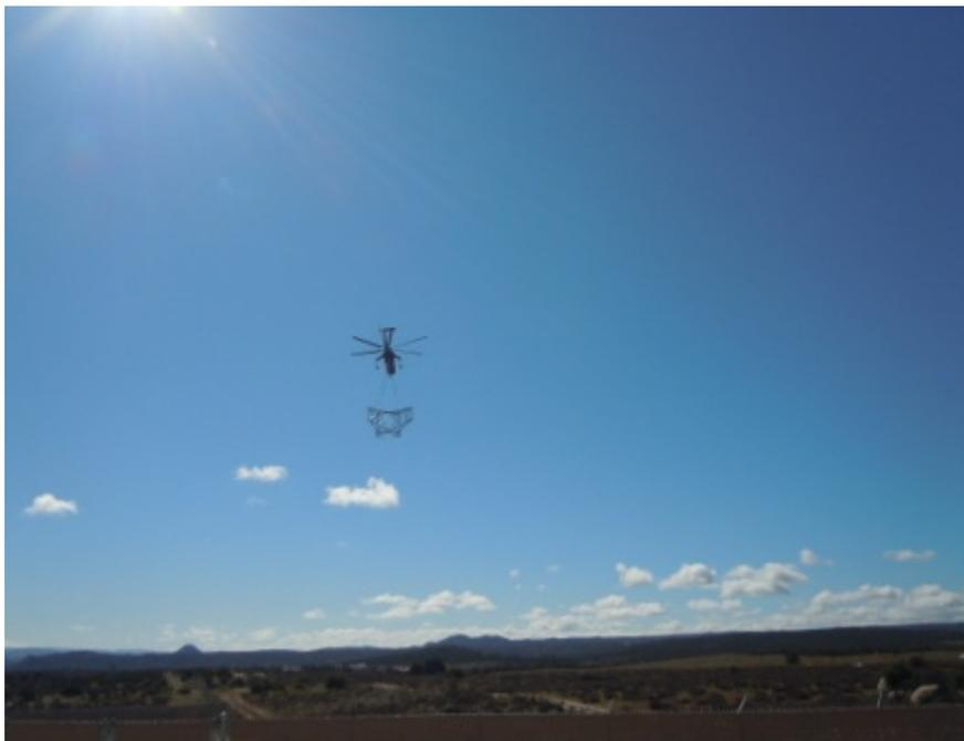
**Figure 2:** The Air Crane is relocating tower pieces within Rough Acres Yard.
