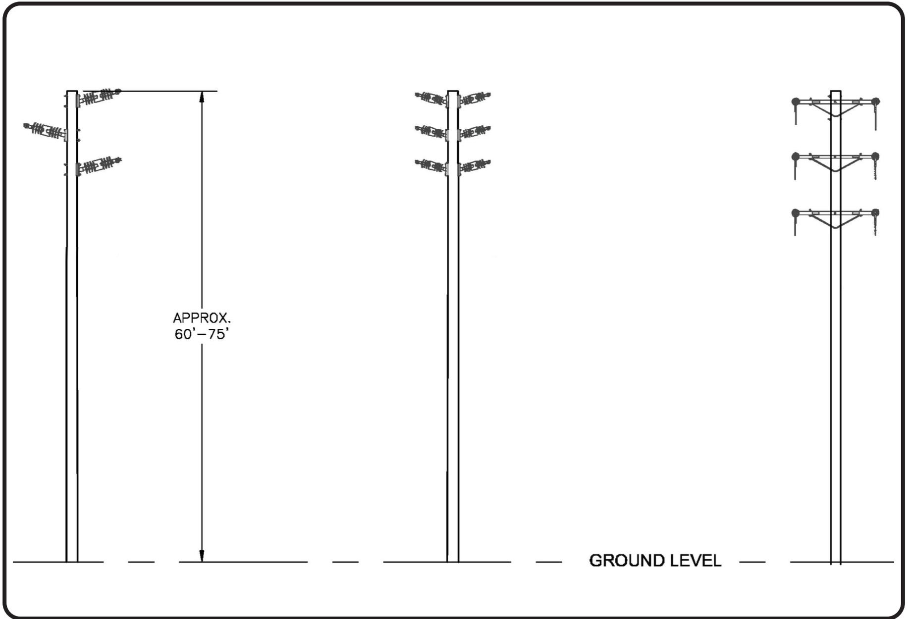
Figure 3-13: Typical Existing 69 kV Wood Pole
