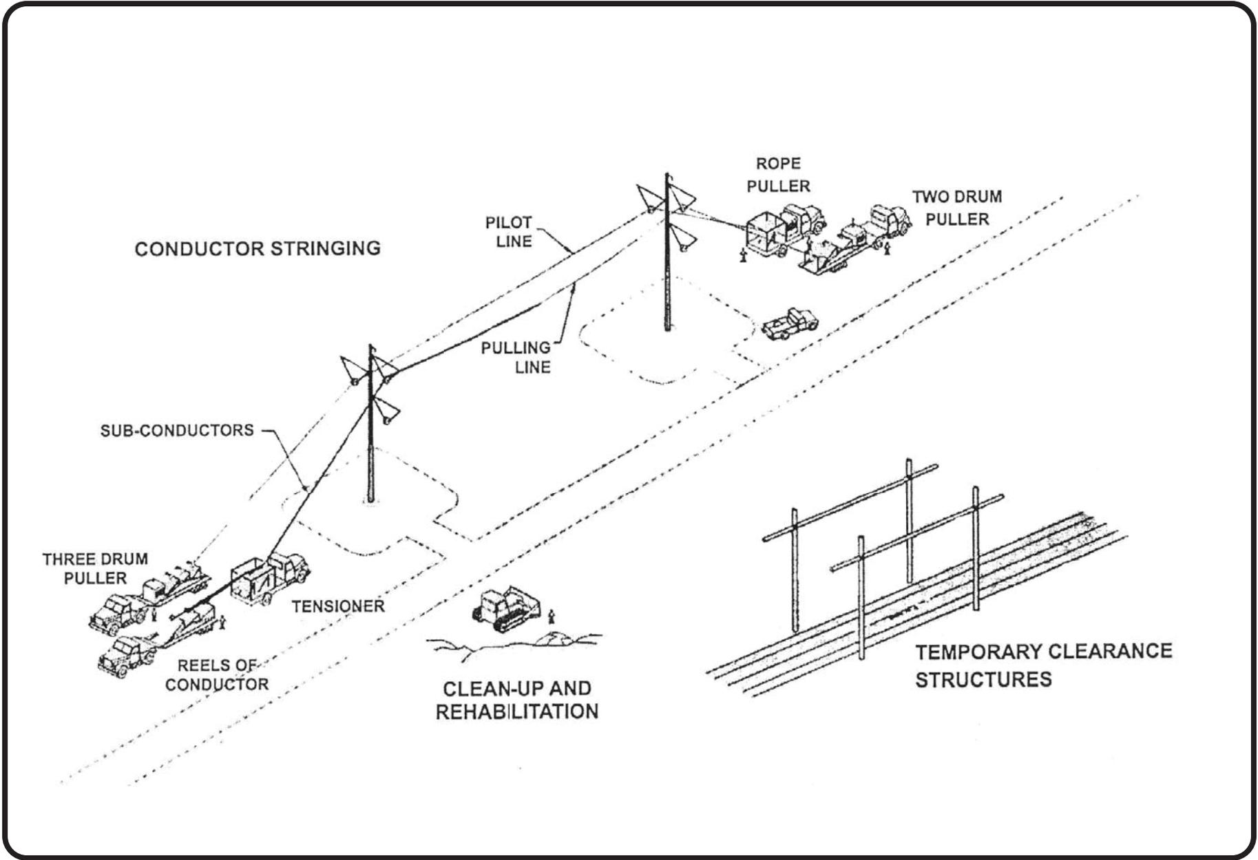
Figure 3-19: Typical Overhead Conductor Installation
