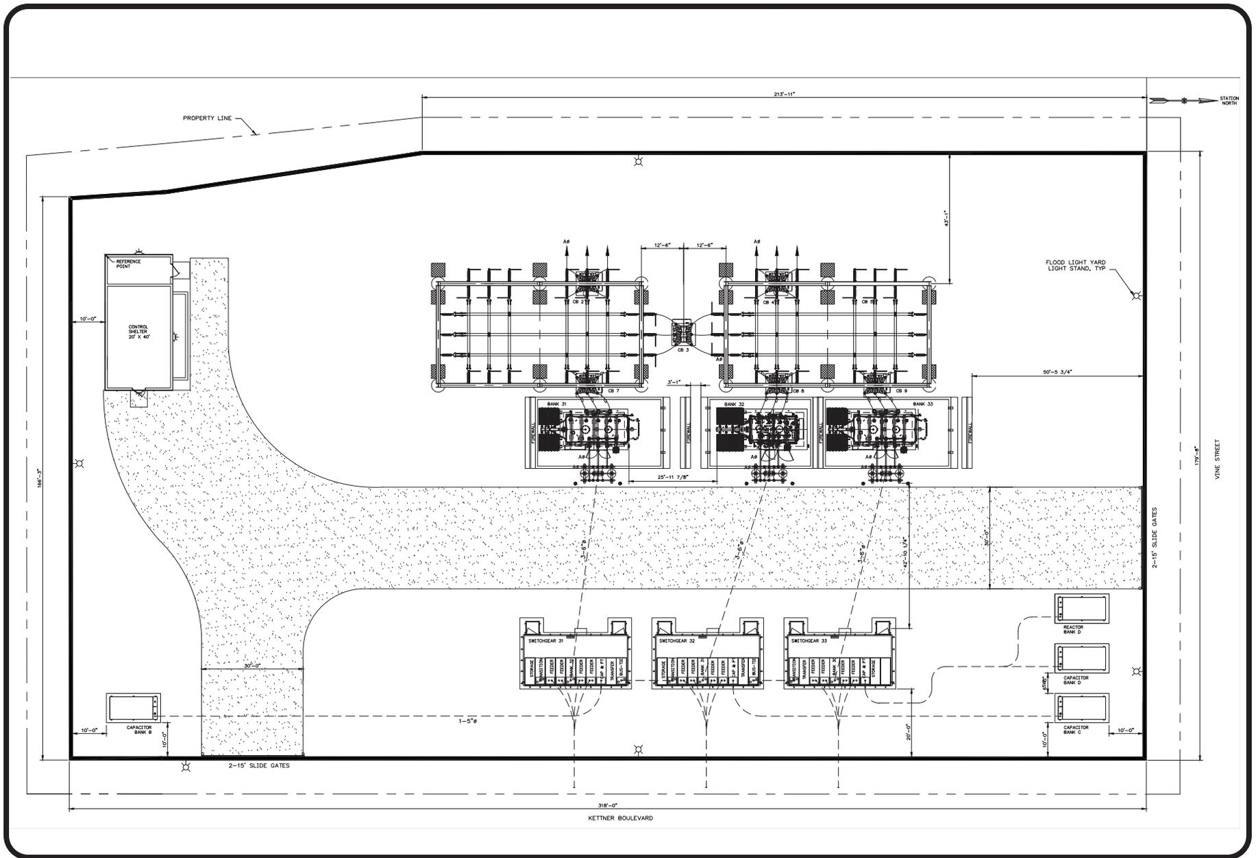
Figure 3-5: Vine Substation Initial Arrangement
