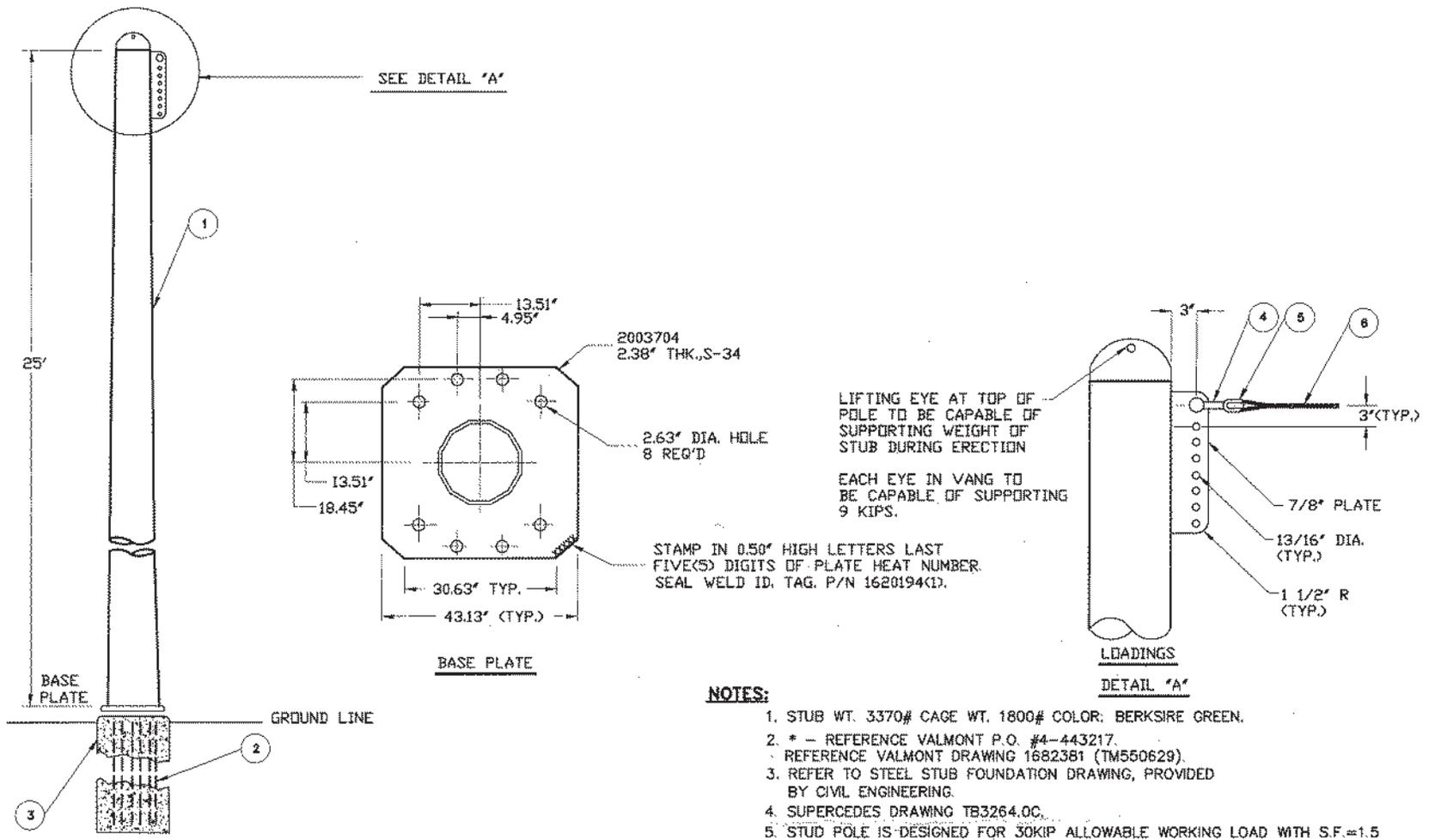
Figure 3-14: Typical Existing Stub Guy Pole
