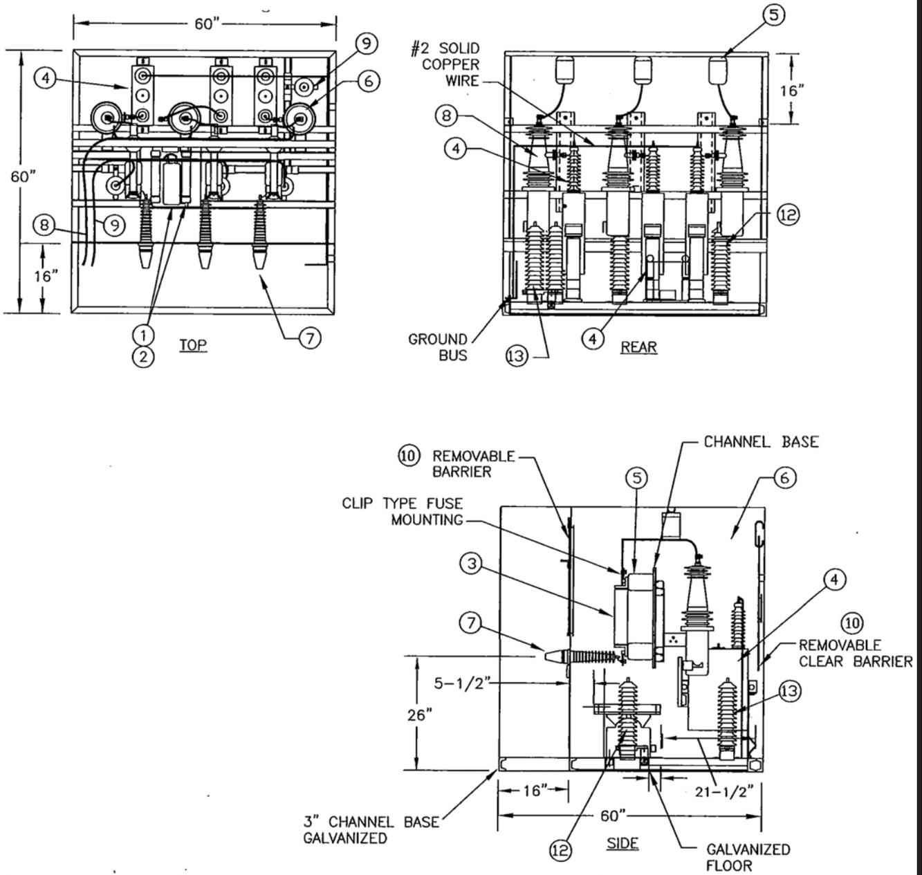
Figure 3-12: Typical 12 kV Capacitor
