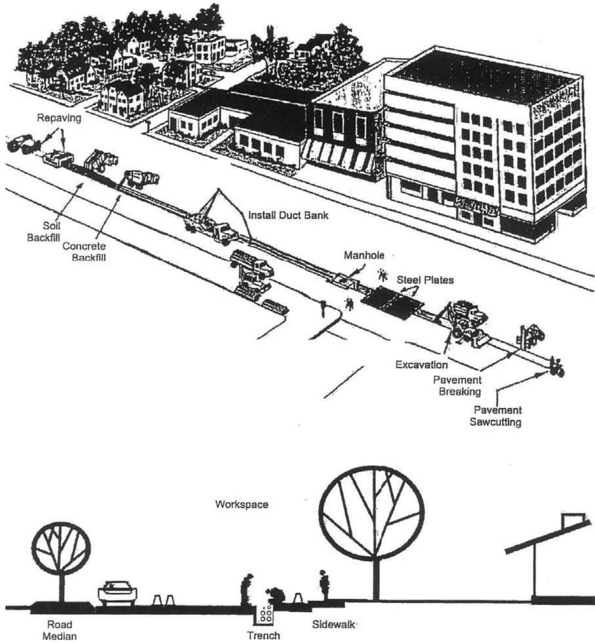
Figure 3-18: Typical Underground Construction Process within Roadways
