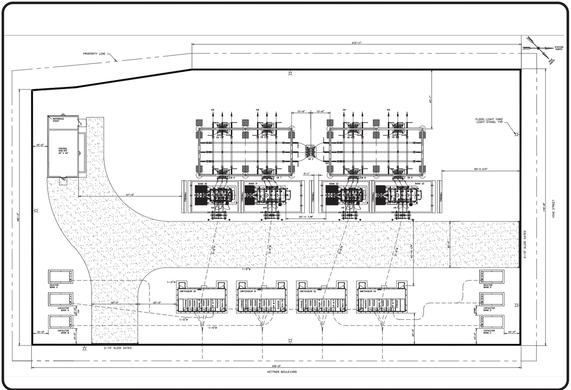
Figure 3-6: Vine Substation Ultimate Arrangement
