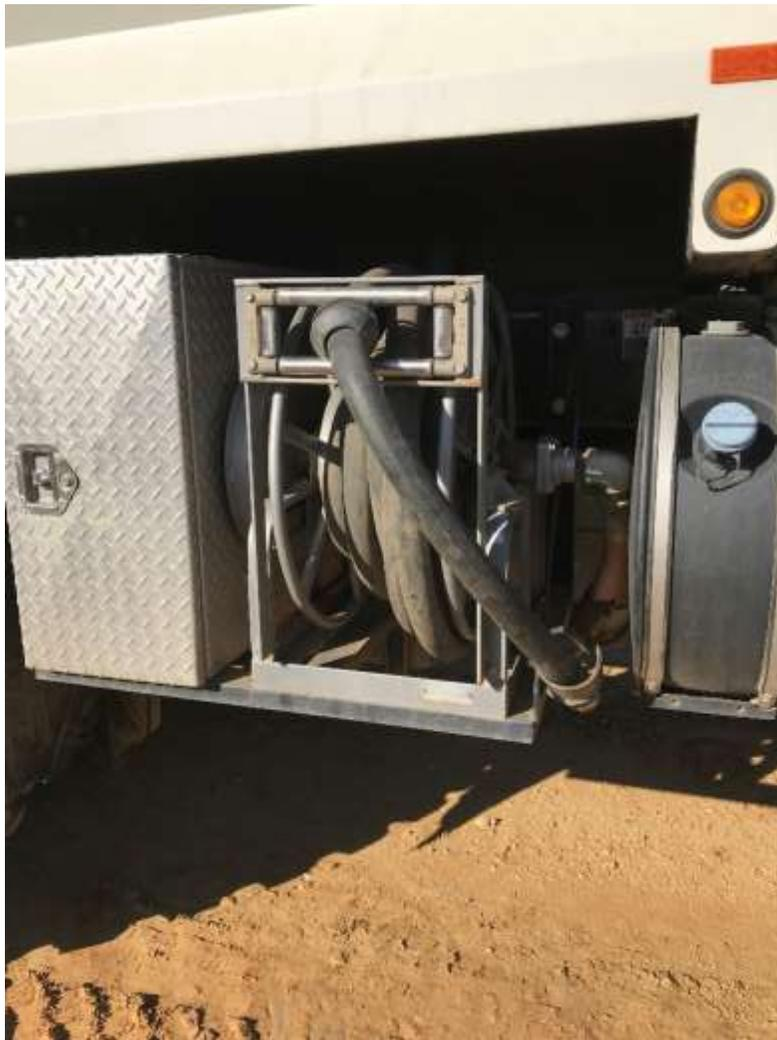
Photo 6 – Insufficient hose on water truck near Palmer Avenue. Per the approved Fire Management Plan, 300-feet of 1-inch hose is required (September 18, 2018).
