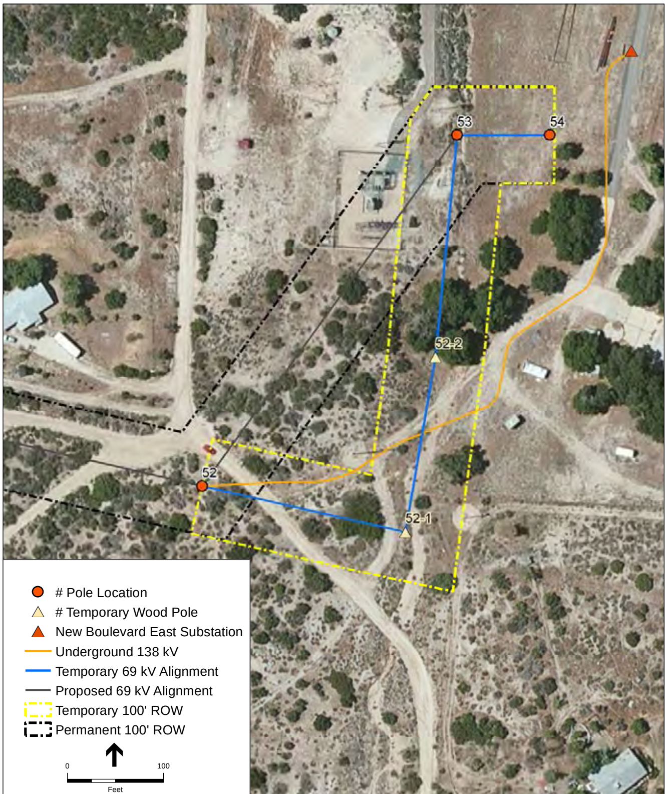
Figure 3-2D Interconnection to Boulevard East Substation - Temporary 69kV Configuration
