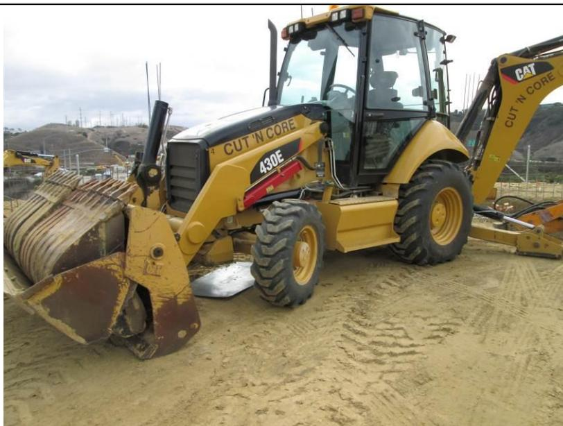
**Photo 4:** In accordance with APM-HYD-1, drip pans were used beneath staged construction equipment to prevent potential leaks from being discharged onto the soil.
