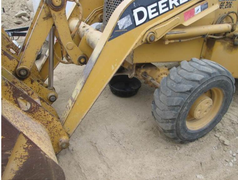
**Photo 5:** In accordance with APM-HYD-1, drip pans were used under construction equipment to prevent potential leaks from being discharged into the soil.
