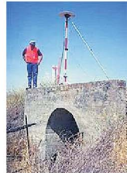
GPS equipment set up at station HERSEY near Colusa Basin Drainage Canal.
