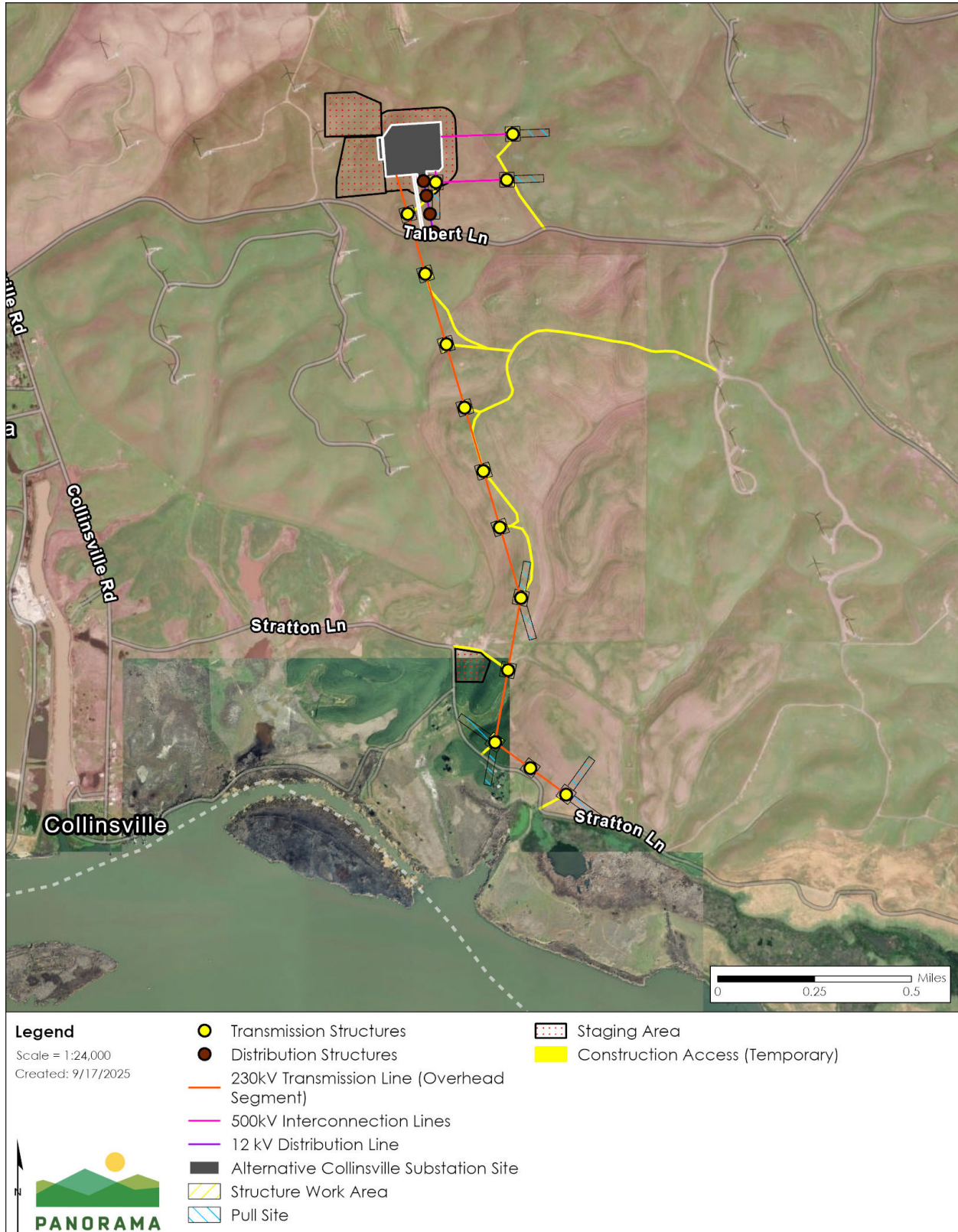
Figure 1 Alternative 1: Collinsville Substation North of Talbert Lane (Retained)
