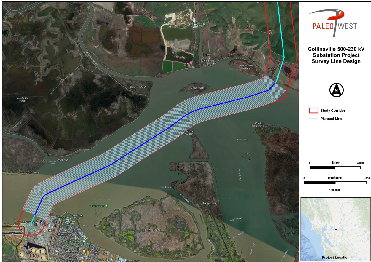
Figure 3. Pre-planned survey lines spaced at 15-meter intervals.
