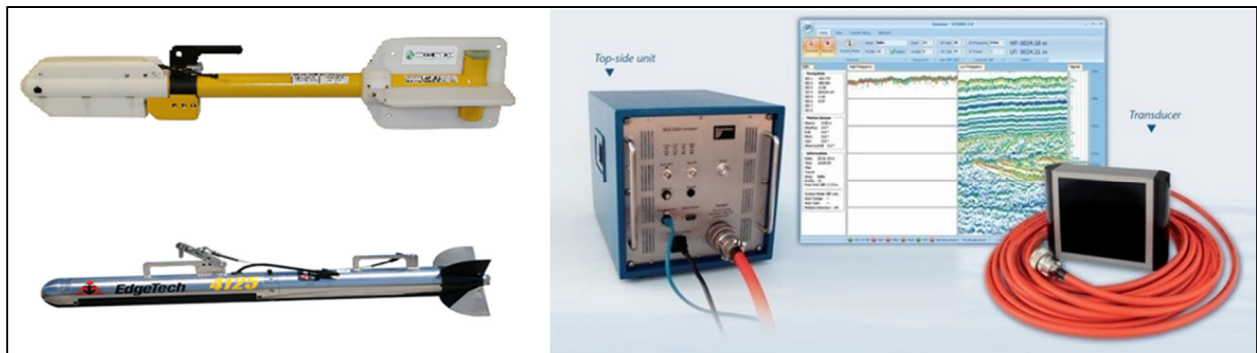
Figure 5-3. Survey instruments employed during the investigation included the magnetometer (top left), side-scan sonar (bottom left), and the subbottom profiler (right).
