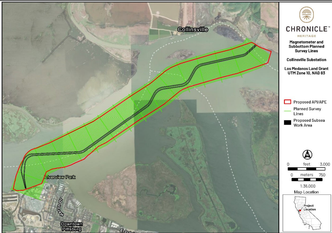
Figure 5-6. Magnetometer and Subbottom 30 meter spaced Planned survey lines.
