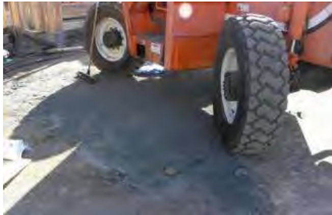
Hydraulic hose leak and absorbent deployment
