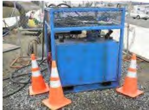
Hydraulic tank leaking onto ground
