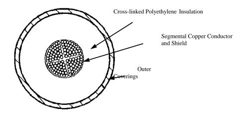
Figure 6 – Typical Cross Section of XPLE Cable
