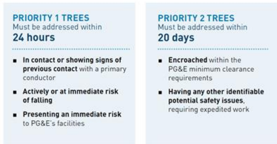
FIGURE PG&E-9.2.1-5: PRIORITY 1 AND PRIORITY 2 TREE TAGS
