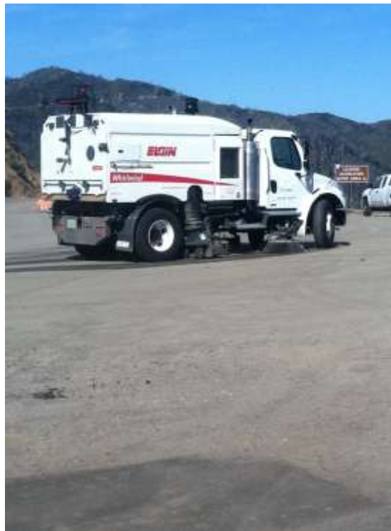
Figure 4: Regenerative sweeper in use on Angeles Crest Highway in response to PM #9.
