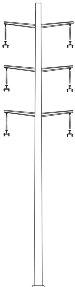
220-kV double-circuit TSP (Height Range: 70-200 feet)
