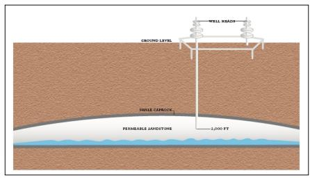
approximately seven miles. Natural gas would be stored in the existing natural reservoir, withdrawn on demand from LGS customers, and conveyed to the PG&E pipeline system for delivery to the customers. The proposed project includes a metering station, gas pipeline, compressor station, flow lines, injection/withdrawal wells, and a temporary gas injection system.
