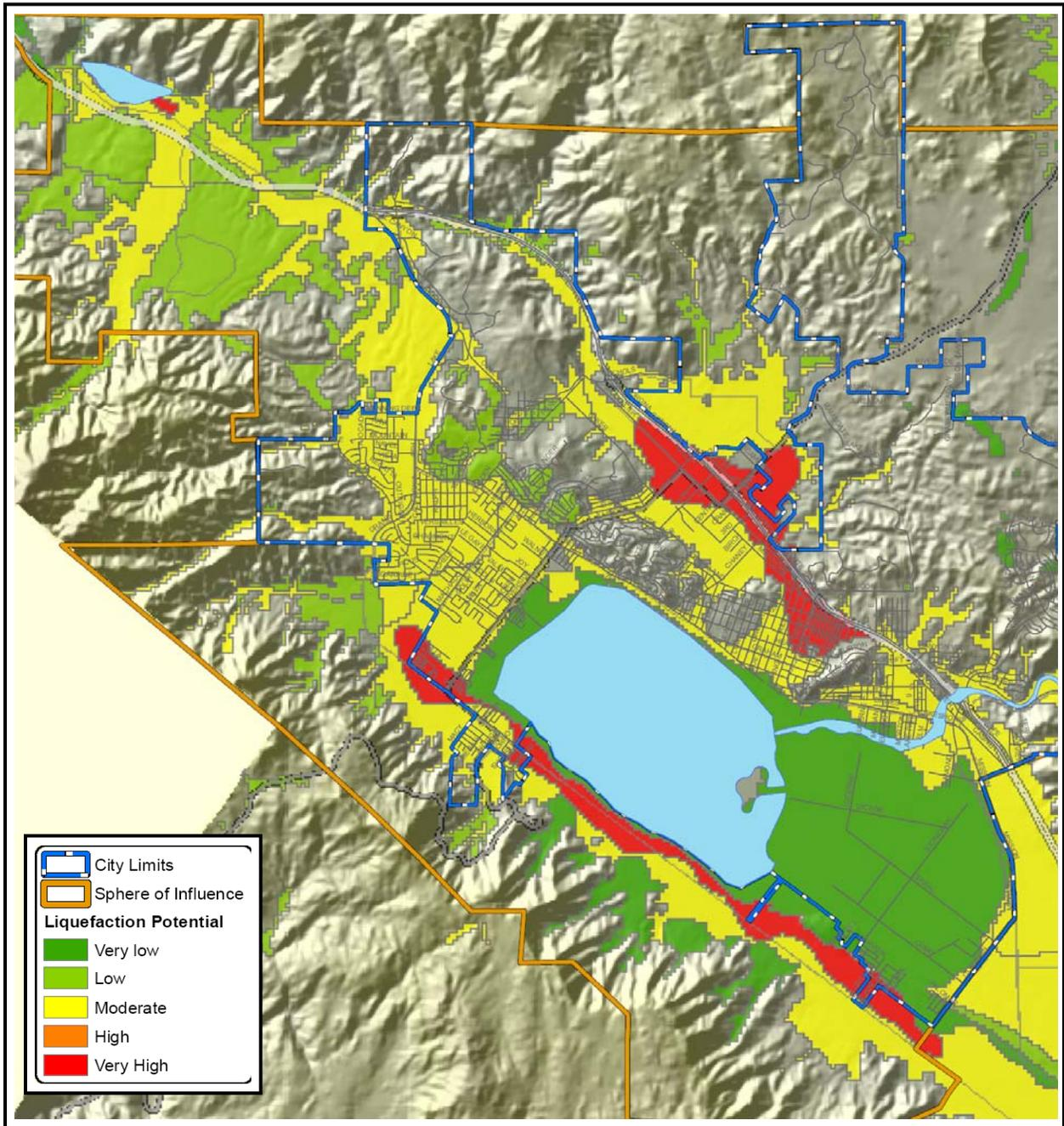
**Figure 4.8.1-4. Liquefaction Susceptibility in the Lake Elsinore Area**
