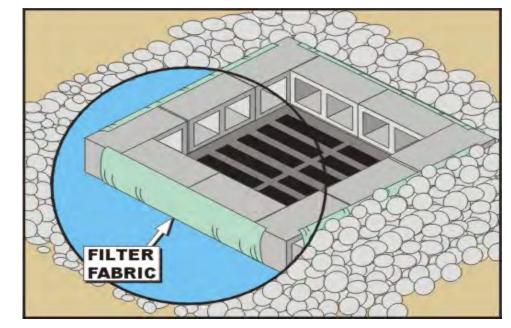
Block and gravel-type inlet protection.
