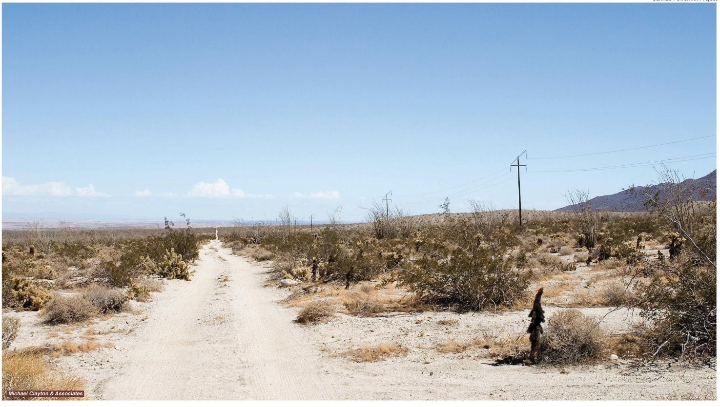
The **existing view** to the east toward proposed structure location SP133 (closest), from Old Kane Springs Road, approximately 0.8 mile east of its junction with SR 78. The vertical forms of an existing 92 kV wood pole transmission line are visible paralleling Old Kane Springs Road to the south (right). The flat, horizontal form of West Mesa is the dominant landform feature. A northeast spur ridge of the Vallecito Mountains is also visible in the right side of the image.
