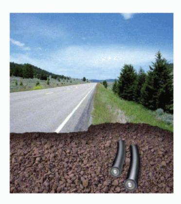
Two 6 inch underground DC cables can provide 4 times the capacity as the overhead Sunrise Powerlink. The trenching depth for underground cables is typically 5 feet by 1 foot in width with a protective cap and no conduit being used for the direct burial cables.
