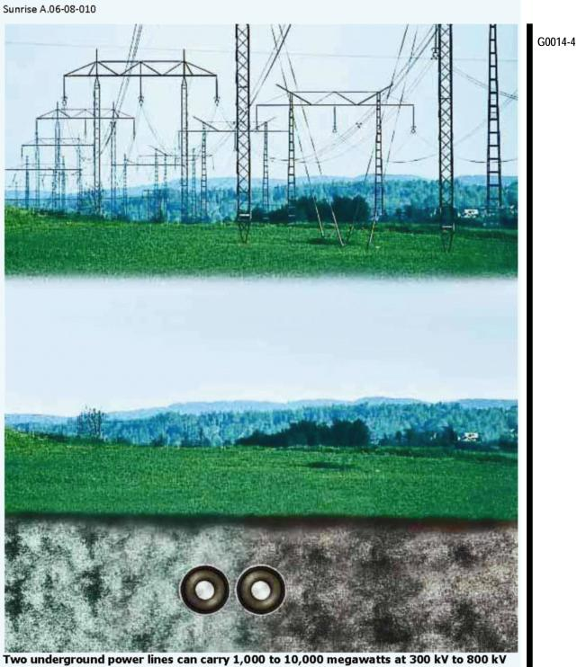
Two underground power lines can carry 1,000 to 10,000 megawatts at 300 kV to 800 kV DC, which is up to 10 times the capacity of the Sunrise Powerlink, all in one small trench, typically 5 feet deep & 1 foot wide, that can be rapidly installed, at lower cost.
