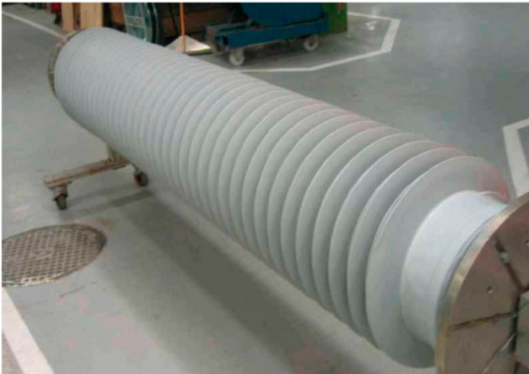
Composite support insulator +-800 kV DC, ABB
