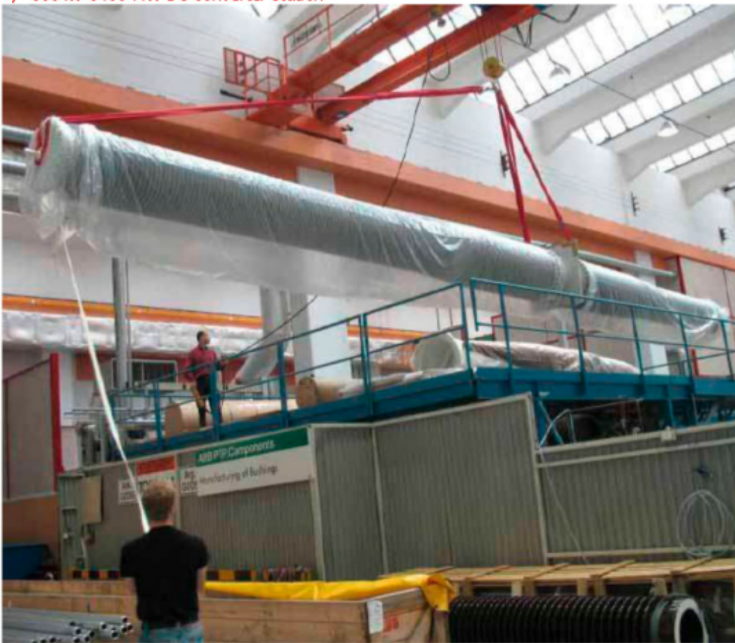
Wall Bushing 800kV ABB
