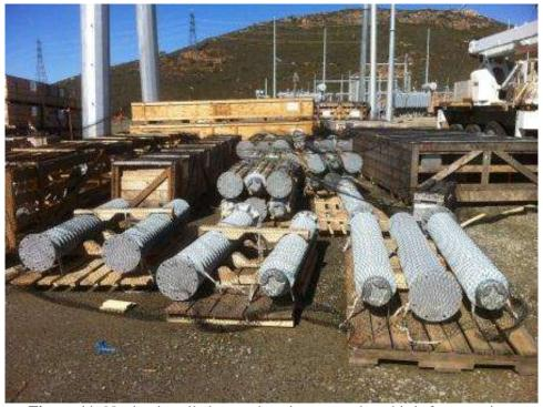
**Figure 11:** Netting installed around equipment to deter birds from nesting. (Link 3)
