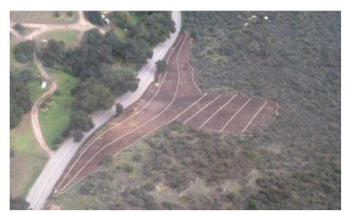
**Figure 6:** Pull site at CP23 with slope restored and BMPs in place. (Link 5)
