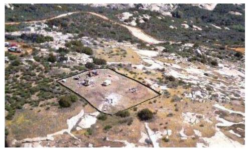
**Figure 5:** Helicopter view of micropile drilling at Tower EP50 with Arroyo Toad exclusionary fencing around the site. (Link 2)
