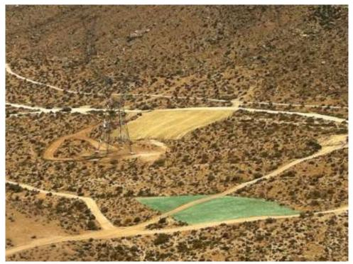
**Figure 1:** Hydromulching at EP255 pull sites. (Link 1)
