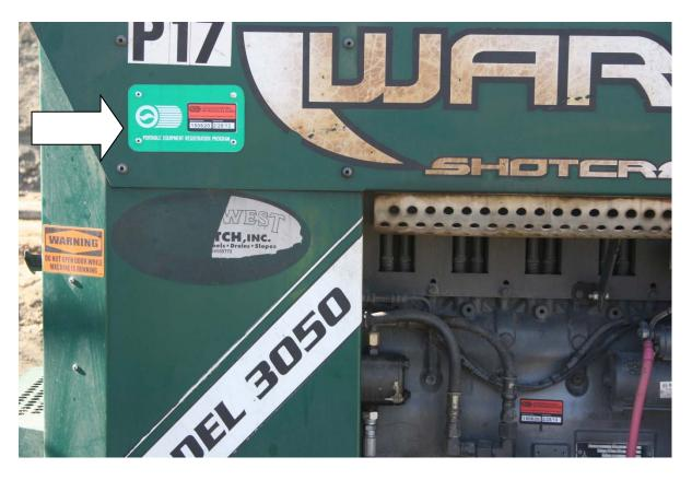
All portable engines 50 horsepower (hp) and above must have a written permit to operate from the local air pollution control district (APCD) or be registered by California Air Resources Board (CARB) under the Portable Equipment Registration Program (PERP). All fuel types are included (diesel, gasoline, propane, etc.). If there is no nameplate or other engine identification, then it must be removed from the construction site if it appears to be over 10 hp.
