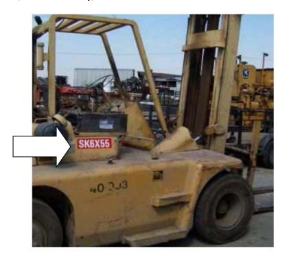
All self-propelled off-road vehicles with diesel engines <u>25 hp and above</u> must be registered by the California Air Resources Board (CARB) under the Off-Road Diesel Vehicle Regulation. Equipment examples include bobcats, backhoes, front-end loaders, graders, forklifts, cranes, man-lifts, and similar self-propelled diesel equipment. If the equipment has no nameplate or other engine identification, then it must be removed from the construction site if it appears to be over 5 hp.
