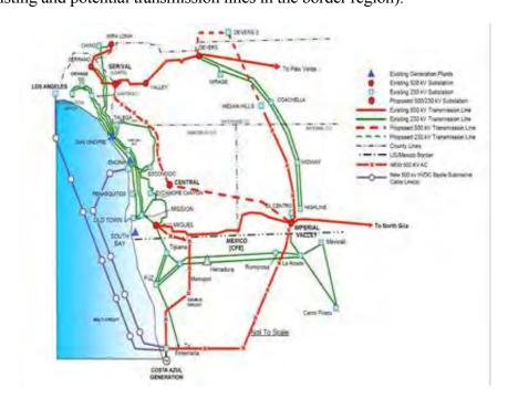
Additionally, East County 69 kV substations and transmission lines would be upgraded to accommodate local wind power development (see inset graphic that depicts the existing SDG&E 69 kV grid). Finally, to improve the reliability of power delivery to the communities of Boulevard and Jacumba and surrounding areas, this alternative would include development of rooftop solar and other local, small-scale energy sources, as well as reinforcement and upgrading of the local energy delivery system.
