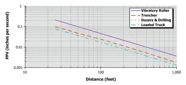
**Figure 8: Construction Vibration Amplitudes**
