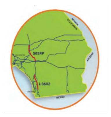
If both the North-South Project and Line 3602 were approved and constructed, the Applicants would have a major 36-inch transmission pathway available to export significant quantities of natural gas from their Northern System through the Southern System to Mexico.<sup>13</sup>
