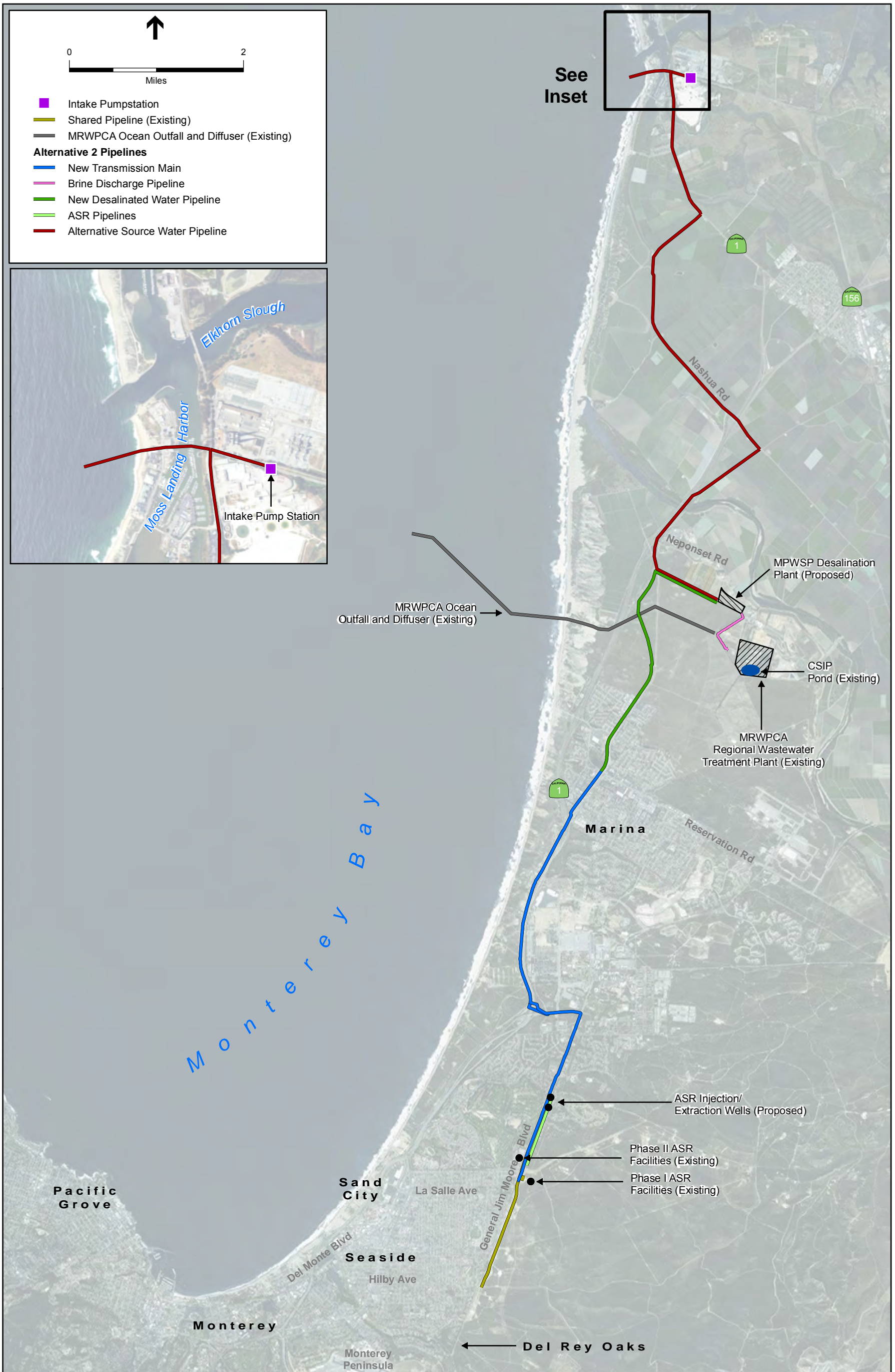
Figure 5.4-2 Alternative 2 - Open Water Intake at Moss Landing
