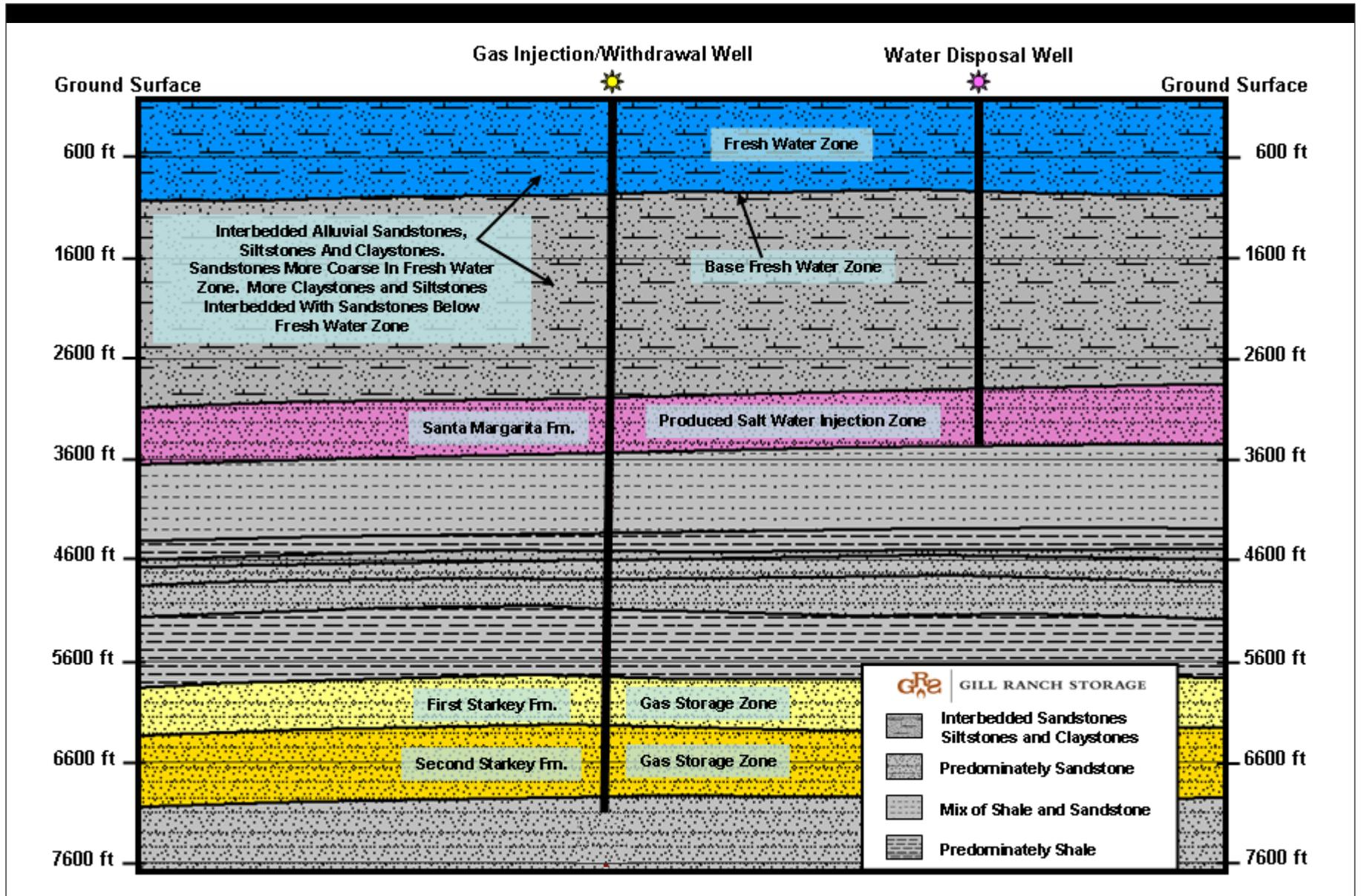
FIGURE 3.5-2 | DIAGRAMMATIC CROSS SECTION THROUGH INJECTION/WITHDRAWAL WELL AND WATER DISPOSAL WELL
