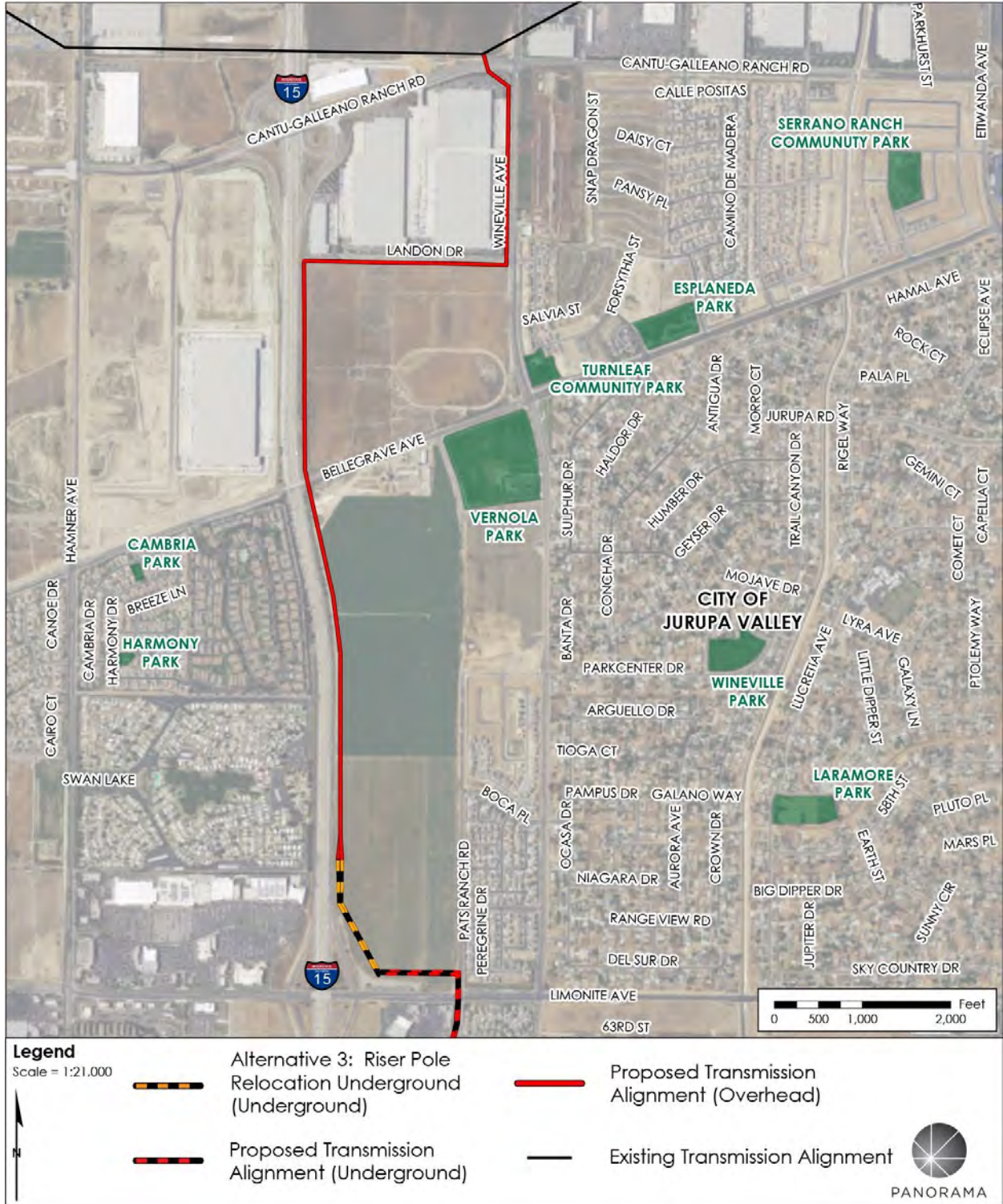
Figure 4.2-3 Alternative 3: Relocate Northern Riser Poles
