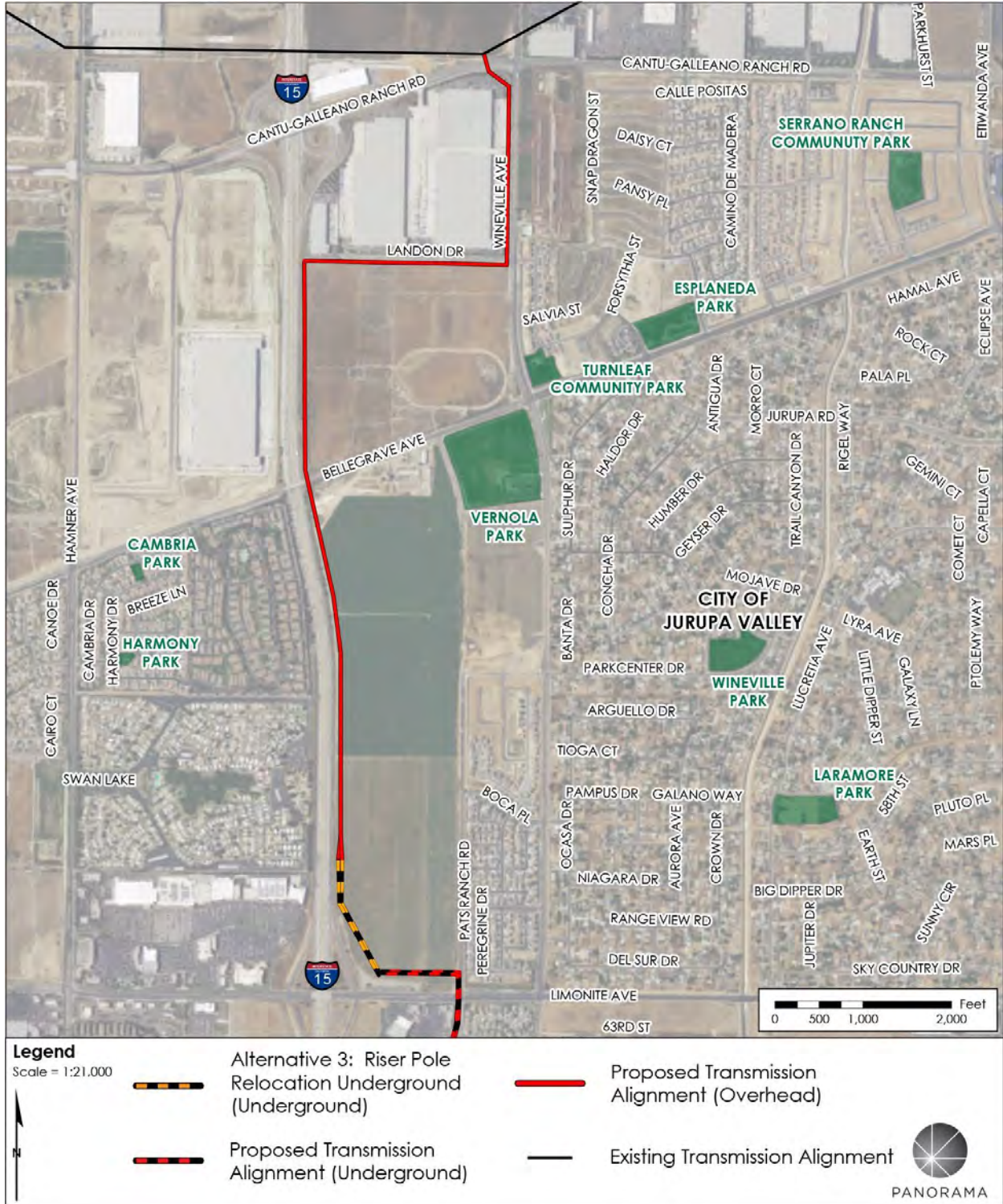
Figure 3.5-3 Alternative 3: Relocate Northern Riser Poles
