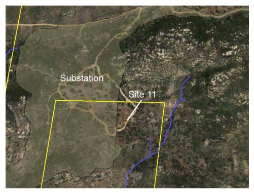
Figure C-20. View of existing road crossing at Site 11 above an ephemeral stream channel and situated on the east-side of the substation (aerial photograph taken 25 May 2009, source: Google Earth, accessed 2010). Present day road-loop alignment seen in the aerial photograph and streams shown in blue. Flow direction is to the southeast from the Site 11.
