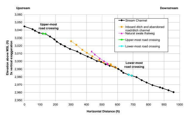
Figure C-15. Longitudinal profile along the intermittent stream channel at Site 1, with flow moving downstream from left to right. The road crossing presently impounds water on its upstream side forming a seasonal pond with wetland vegetation.
