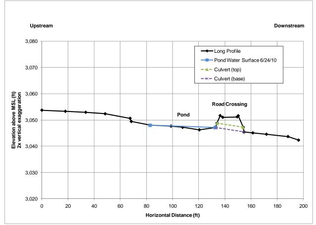
Figure C-6. Longitudinal profile along the intermittent stream channel at Site 1, with flow moving downstream from left to right. The road crossing presently impounds water on its upstream side forming a seasonal pond with wetland vegetation.
