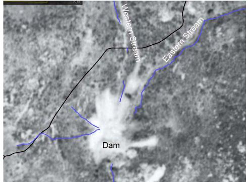
Figure C-24. View of historic road, stream, and dam alignment at Sites 2 and 3 (aerial photograph taken 2 Apr 1953). Present day road alignment shown in black and streams shown in blue. Note the roadway to the west and the road crossing were not present (constructed 2002-2003).
