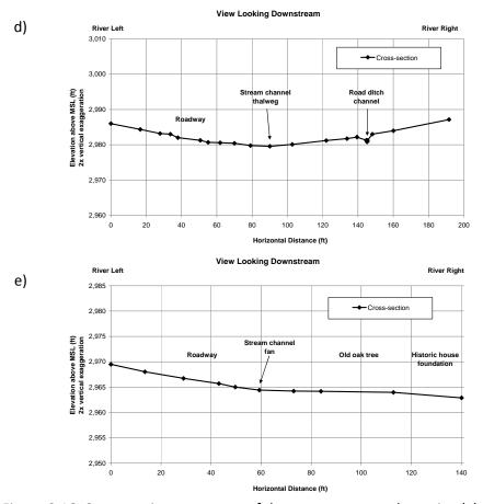
Figure C-16. Cross-sections upstream of the upper-most road crossing (a), upstream of the confluence with a natural ephemeral swale confluence and the proposed stream and ditch channel confluence (b), downstream of the proposed stream and ditch channel confluence (c), downstream of the lower-most road crossing (d), and across the fan of the stream channel at the upstream end of the southwestern meadow.
