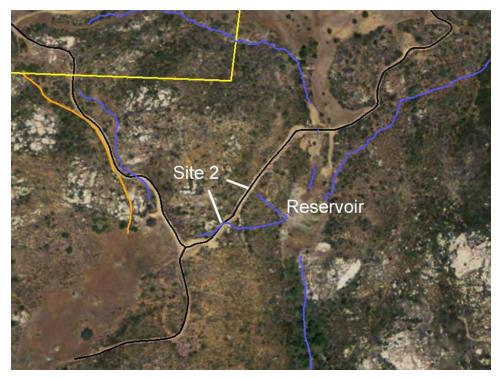
Figure C-17. View of existing road crossings at Site 2 along two ephemeral stream channels that drain eastward to the large reservoir (aerial photograph taken 25 May 2009, source: Google Earth, accessed 2010). Present day road alignment shown in black and streams shown in blue.
