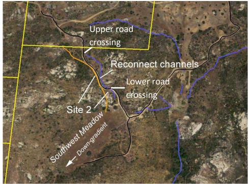
Figure C-9. View of existing road crossings at Site 2 along the stream channel that drains to the southwest meadow (aerial photograph taken 25 May 2009, source: Google Earth, accessed 2010). Present day road alignment shown in black, abandoned road and ditch shown in orange, and streams shown in blue.
