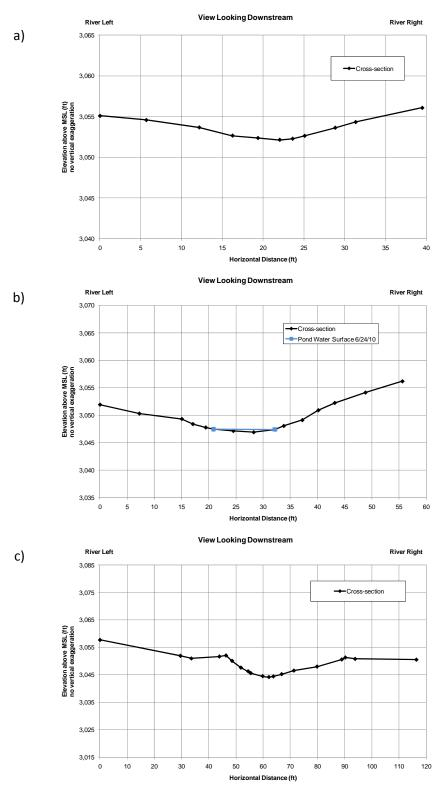
Figure C-5. Cross-sections upstream of the road crossing (a), across the pond upstream of the crossing (b), and downstream of the road crossing (c).
