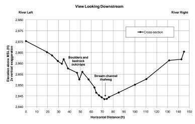
Figure C-30. Cross-section of the stream channel downstream of the large reservoir dam. Boulders and bedrock outcrops are present on the river-left upland slopes and the dam spillway is present in the notch near the top of the river-right upland slope.
