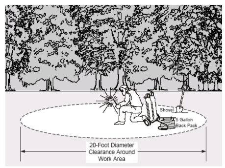
Proper clearances around welding operation.
